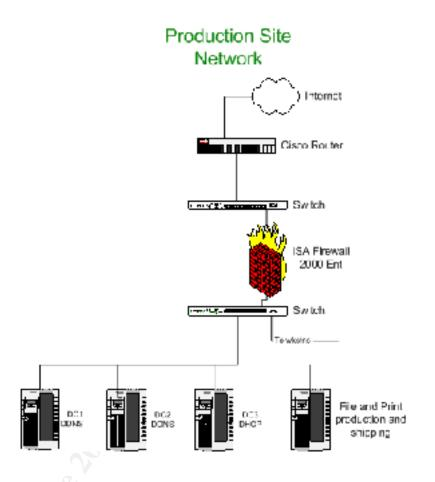
Our production site network (figure 2) will contain the following servers, all of which will be our standard hardware setup with five disk RAID 5 arrays;
