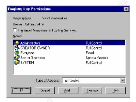
One reason for setting the permission on the registry key is because of other NT vulnerabilities that may not have been controlled. For example, remote access to the registry may still be possible, in which case allowing Everyone to have read access is giving it to anyone, authenticated or not.
