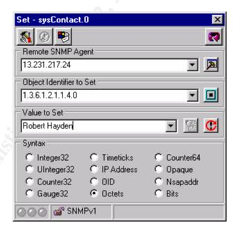
should be noted that a graphical interface was used to easily locate the contact information field (shown as sysContact.0) in the header bar at the top of the figure. Other information is just as easily located, such as computer name.
