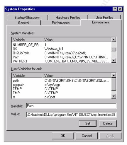
Reboot the machine. Now, NTList is ready for use. Increasing the command line buffer size is also useful but it is not required.
