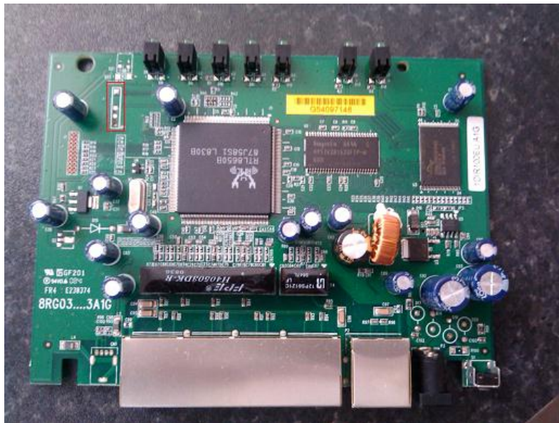
Figure 7- Potential serial pins highlighted in red square
