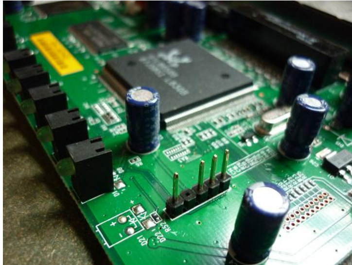
Figure 8 – Pins soldered for serial access
