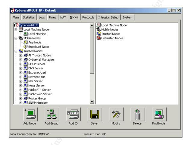
The Add Node button brings up a dialog box that will allow the user to edit the node name and IDs. The Add ID, Delete ID, and Modify ID buttons allow the user to change the IDs for the node. Selecting the add button brings up the following dialog box:
