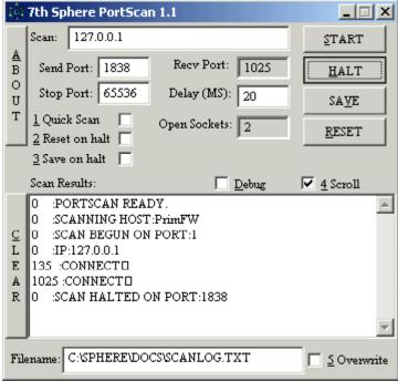
After running port scans against the various servers in the DMZ and in the internal networks, the logs of the firewall should be checked. The logs should list all illegitimate attempts to connect to various machines.
