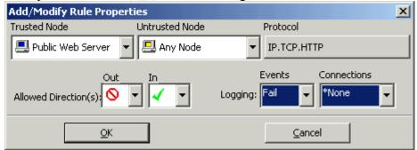
All options are available in a drop down box except the Protocol option. This opens another dialog that allows the users to select what protocol to use. After clicking the OK button, the rule is added to the rule base as shown below.
