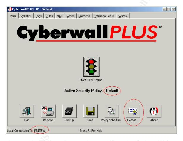
The Remote button will allow the user to change to a different firewall to be modified. The user has the option of using encryption or not.
