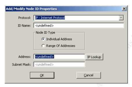
This is where individual nodes or subnets are created. With an individual node the subnet mask option is grayed out. When selecting a range is it important to get the correct subnet or misinterpretation of the rules could result.
