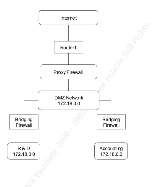
This solution assumes a public address space of 198.198.0/24 and an internal, private address space of 172.18.0.0/16. To provide the greatest security for the two subnets we will need to layer our defenses and isolate the physical subnets.
