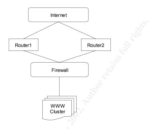
The two lines (each from a different ISP) connecting the Internet to the routers are DS3 (45 MB lines) choked down to only 6 MB/s each. Each line is subscribed to with the ISP as burstable lines. This means that when the traffic exceeds 6 MB/s on that link the line will continue to operate up to 45 MB/s. This means that a DDOS attack must sustain 90 MB/s to saturate your Internet connection.
