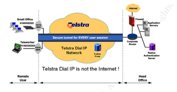
Sample diagram of Telco provided VPN tunnelling:
