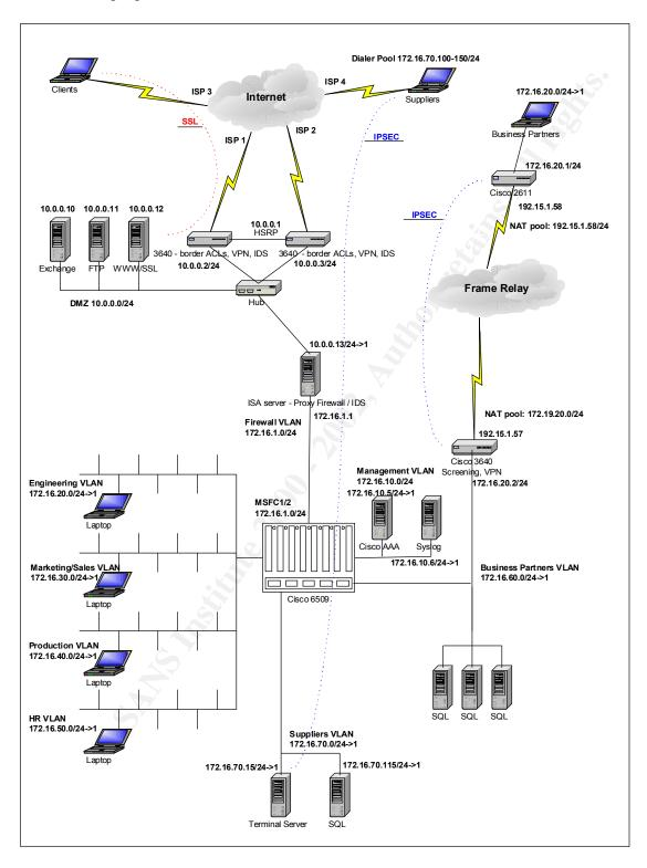
The border router consists of two physical boxes (Cisco 3640) running Cisco Hot Standby Router Protocol (HSRP) for the purpose of redundancy and recovery from DDOS attacks. Some actions were planned and done to minimize the impact of possible DDOS attacks, but in some cases the system will not be able to defend and will eventually go down. This design offers two T1 connections to two different ISPs, there is no load balancing, one link is in hot stand by state (passive) and another is active.
