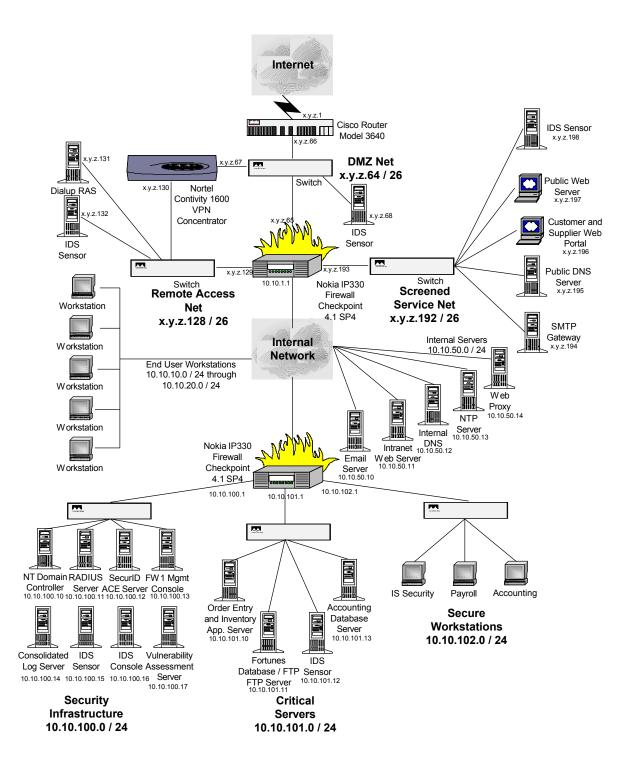
All servers on the DMZ, Screened Service Net, and Remote Access Net are running Slackware Linux 8.0 with Kernel 2.4.9. These servers have been appropriately hardened for service as bastion hosts. The DNS server is running Bind 8.2.5, the Web Servers are running Apache 1.3.22, and the SMTP gateway is running Sendmail 8.12.1 and Interscan Viruswall 3.6 with updated scan engines and virus signatures.
