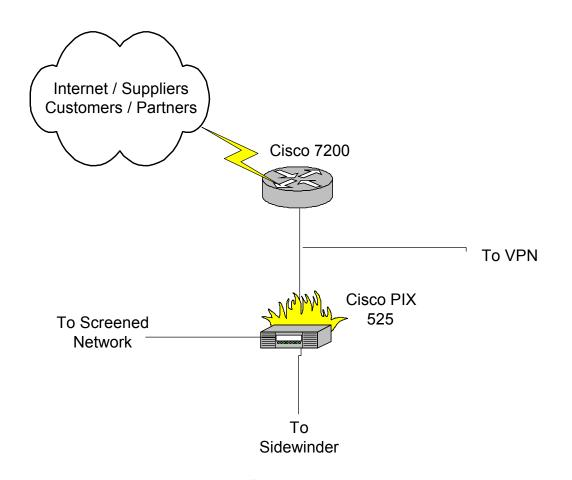
The first module in SAGE is the "Badlands" module. This is the outermost section of the GIAC Network and through this border router is the primary point of connection for all data entering the GIAC Network from untrusted sources, namely the Internet.
