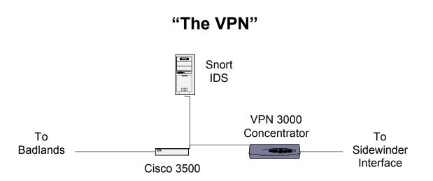
The VPN segment of SAGE contains a Cisco Catalyst 3512XL Switch, a computer running SNORT as its Intrusion Detection System software, and the Cisco VPN 3030 Concentrator providing the VPN services to the GIAC Enterprises, Inc. partners.
