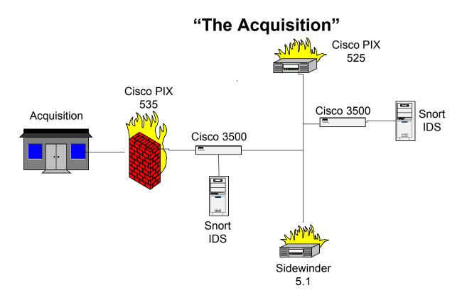
The Acquisition module of SAGE consists of two Cisco PIX 535 Firewall devices, one at the Acquisition location and on site at GIAC Enterprises. The two Firewalls are connected across a T-3 line as a Site-to-Site VPN using IPSec. GIAC Enterprises will provide all of the Internet connectivity needs of the acquired company, i.e. e-mail, Internet browsing, etc., through this VPN connection.
