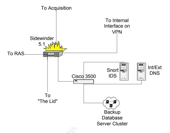
The DNS/DB Zone consists of the usual Cisco 3512XL and the Snort IDS Server, but in addition is an Internal/External DNS server which is the second of three DNS servers used to implement a split/split DNS architecture. The split/split DNS Architecture increases your protection from an attacker who attempts to poison the DNS cache of your DNS servers by shielding the Internal DNS from the External DNS.
