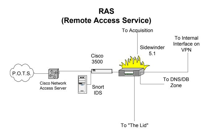
The RAS module of SAGE was set up to establish a method of connecting corporate users to the GIAC Network without them having to dial an Internet Service Provider and enter via the VPN. A Cisco Network Access Server is utilized as the authentication mechanism for users that dial in. Also located in this segment are the usual Cisco 3512XL and the SNORT IDS Server.
