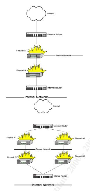
We can mitigate this risk by configuring firewalls in series so that both must be compromised before the internal network is reached. If different firewalls are used for the two layers then no single vulnerability will result in security being breached. However, either firewall is now a single point of failure that would result in the system being offline.
