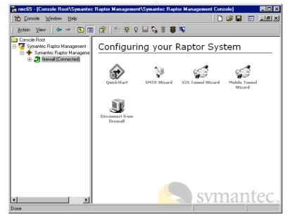
This screenshot shows the scope pane with the management directory tree fully expanded. The next stage of configuring the system is to work through the Base Components, configuring each in turn.
