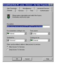
The General tab allows a description to be given of the rule, the interface through which traffic comes in and out of the firewall server and the source and destination network entities.
