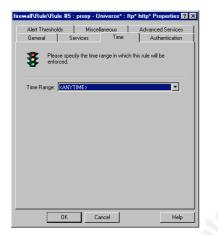
The time tab allows the time to be set for which the rule is active. Most of our rules will be set to be permanently active: <ANYTIME>
