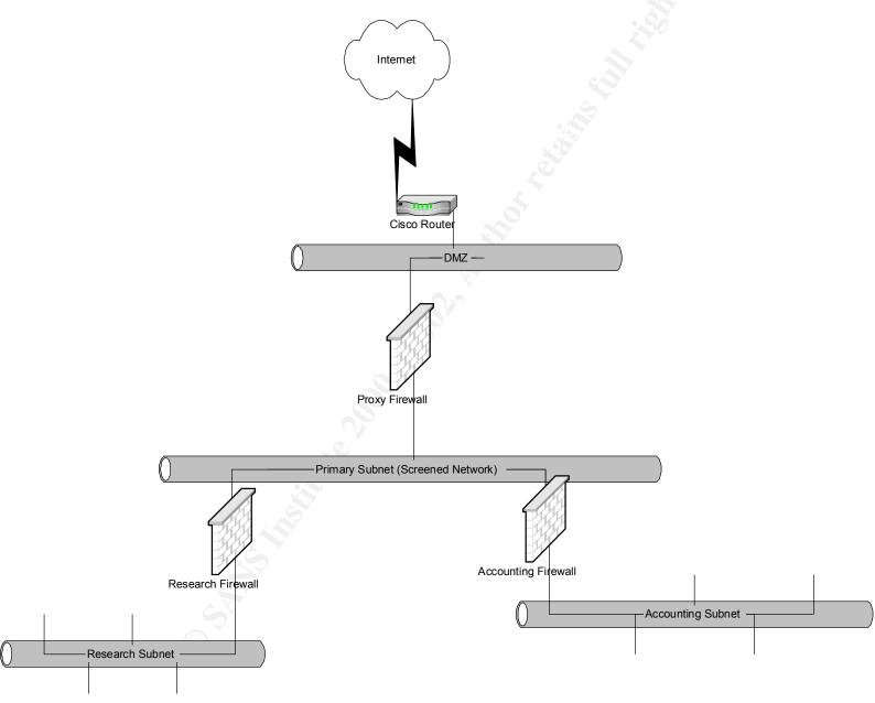
First, we will want to setup the Cisco Router as our Border Gateway router. We will connect the serial interface to the line from our ISP and the Ethernet interface to our DMZ. The DMZ will contain our valid address space. On the Border Gateway router, we will want to perform Egress filtering as well as denying all reserved address spaces (RFC1918).
