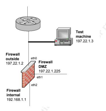
The test machine's operating system is Linux RedHat 7.2 - kernel 2.4.9-21. The following default route is added to the test machine to make sure that the traffic goes the correct direction:
