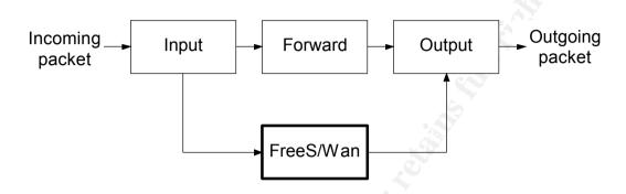
FreeS/Wan is running as a local process and has its own "network interface" called *ipsec[number]* ( ipsec0 in GIAC's firewall). This interface is treated in the same way as the *eth[number]* interfaces by Netfilter, i.e. using INPUT, OUTPUT and FORWARD chains.
