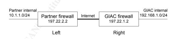
FreeS/Wan uses the naming conventions "Left" and "Right". The shown settings above are used in the configuration files (see 3.3 - Configuration files).
