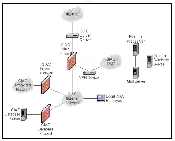
Notice that the VPN device is placed between the firewall and the GIAC DMZ. This architecture offers several advantages:
