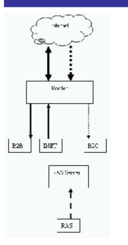
For performance reason, a minimum of two internet links are deployed, with one devoted to servicing the customers (B2C) and the other one for servicing access requests from external partners and suppliers (B2B) as well as outgoing internet requests made by the internal staffs (INET). RAS access (RAS) is made available via direct dial in, and has nothing to do with the internet.
