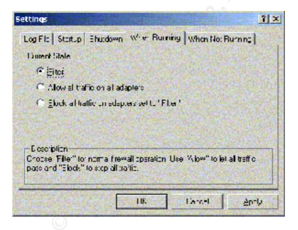
When the firewall service is not running (or is not YET started), all traffic should be blocked.
