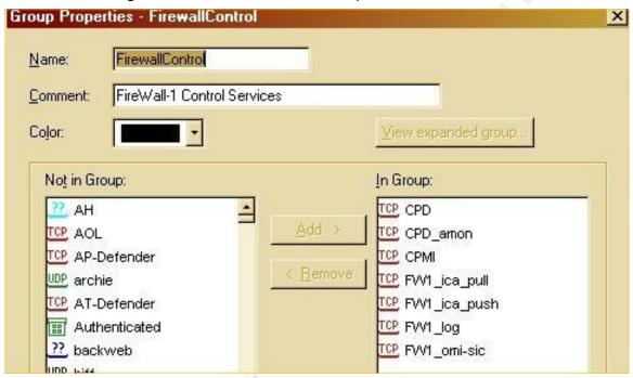
We also create a group that contains the IP addresses of the IT staff's workstations and VPN IP address pool for the purposes of connectivity to the management station. To create a group of network objects we select Manage → Network Objects → New → Group:
