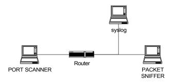
We will port scan both the router and the packet scanner to insure that we have sufficiently harden the router as well as blocked the appropriate ports. The packet sniffer will used to verify that the ports are being blocked and the logging to syslog is working.
