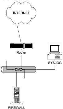
The router is the first line of defense in a multi-layer approach to perimeter security. The router will augment the firewall, which is our main defense against attack, by blocking the ports that are commonly used in probes and attacks. This approach will stop the majority of the script kiddies but it will only slow down a determined intruder from probing and attacking the firewall.
