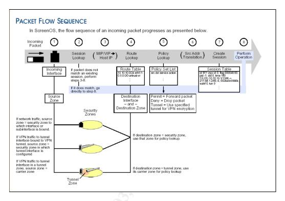
When access rules are created, the Netscreen implicitly creates corresponding rules allowing replies to service requests. For example, a policy allowing HTTP traffic from the Internet to the web server on port 80, will result in an implicit rule allowing the reply traffic back out, based on state tables the Netscreen maintains and uses to remain aware of session states.
