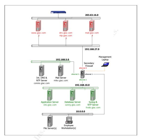
A dedicated server management PC is used to remotely manage servers in all zones. This PC is physically secured at GIAC's premises and cannot be connected to remotely. Physical access to GIAC's premises is required for server management.
