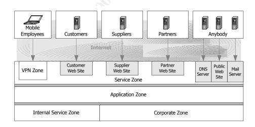
The diagram above illustrates the logical separation of GIAC's IT resources into security zones. A zone is a collection of resources which is protected from other zones. In this case, zones represent GIAC's different networks and are protected by a combination of packet filter ACLs and firewalls.
