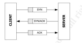
As we can see from the diagram, in a normal TCP connection, the client sends a SYN packet to request a connection, the server acknowledges the request with a SYN ACK, then the client acknowledges that with an ACK of its own. From that point on, the connection is established and data can now flow.
