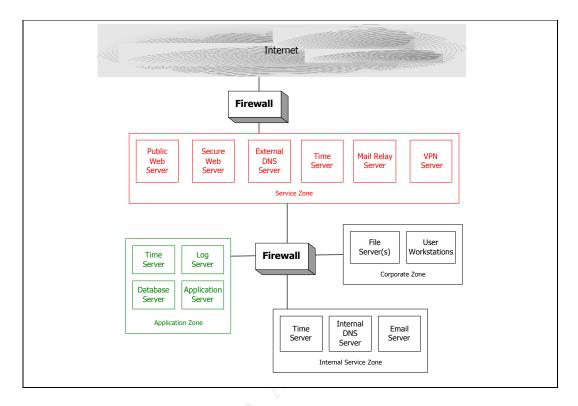
The logical architecture depicts what functional components exist and how they are grouped into logical zones. The lines show which items are connected, but it does not represent the direction of communication or the method of communication.
