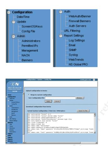
As the menu structure shows, there are a wide range of system options configurable through the Netscreen GUI interface.
