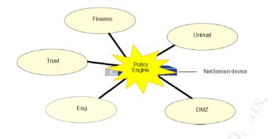
A zone is applied to a physical network interface, enabling the Netscreen to control traffic between zones. Security zones are logical objects, so it is possible to define more than one zone on a single physical interface.
