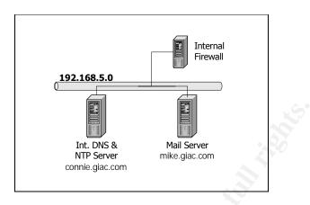
The internal service zone hosts the mail server, internal DNS server and an ntp server. The ntp server synchronises time from ntp.giac.com and acts as ntp server for the rest of the network and the DNS server answers all GIAC's internal DNS requests.
