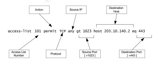
An example of [options] would be to add log at the end of the command, telling IOS to log matches to the rule, whether locally or to a syslog server.
