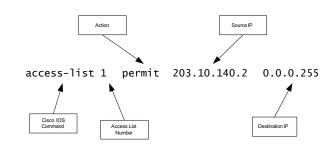
This example permits any traffic from any host on the network 203.10.140.0. The zeroes in the destination IP must match the corresponding octet in the source IP and 255 means that the fourth octet does not need to match. Whilst a standard ACL would be adequate for blocking invalid source IP addresses, GIAC needs a more sophisticated filtering capability to enable filtering of traffic to the service zone and the VPN.
