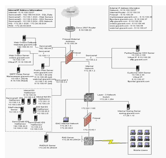
Greg's design employs a Symantec Enterprise Firewall v7.0, running on a MS Windows 2000 Server with Service Pack 2 installed.
