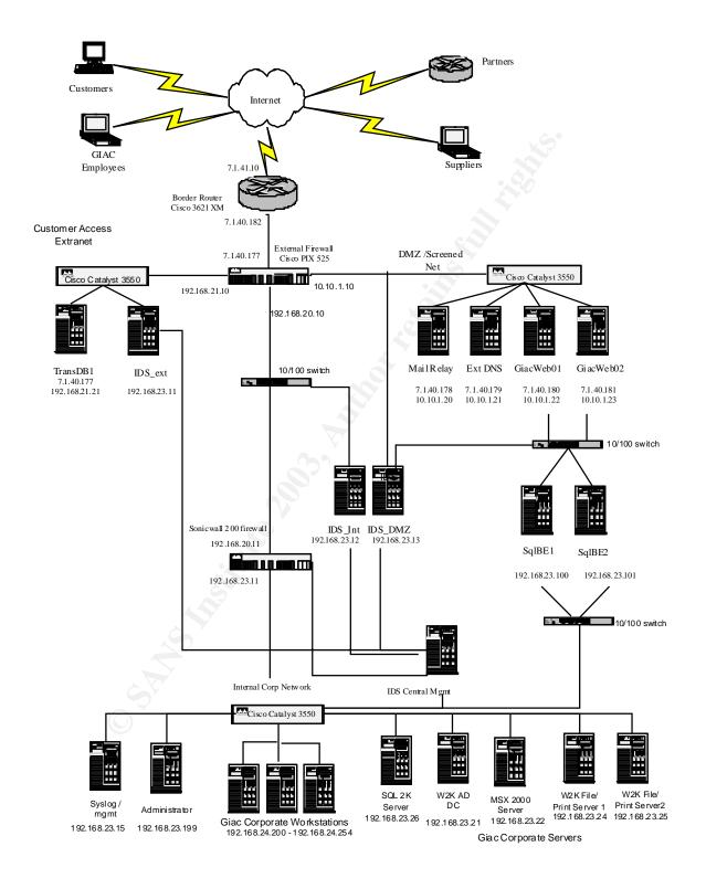
The components included in this architecture represent Defense in Depth, which is achived by implementing a layered approach to security. Each device performs its own security functions in conjunction with each other device. However, when the devices are taken as a whole, they represent a layered security design.
