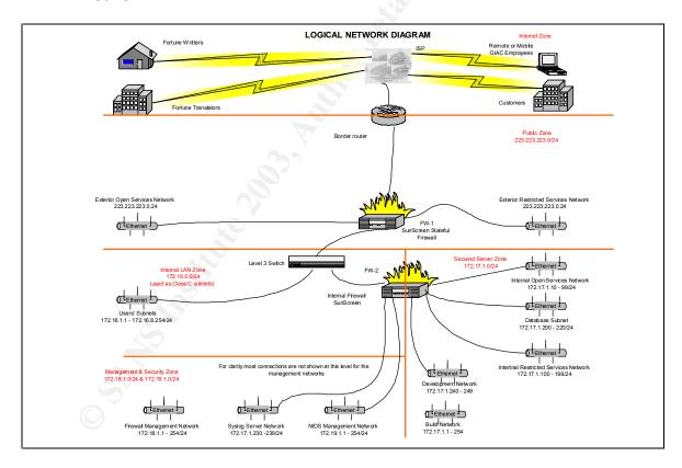
The boundaries of the security zones have been created by the insertion of a firewall and filtering routers. Most security subnets are created by attachment to a port on a firewall. The multiple user subnets, which are collectively a security zone, have been created as multiple VLANs on a Cisco 6506 level 3 switch. We have chosen this switch because of its proven track record, expandability and feature rich software
