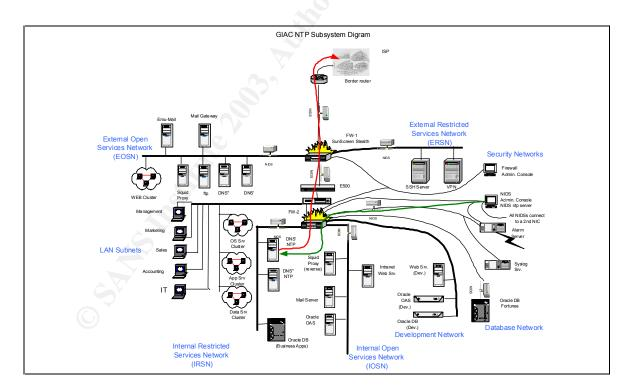
The ntp subsystem uses three ntp servers. The two primary ntp servers are co-hosted on the two internal DNS servers. Only these two ntp servers are permitted to request updates from four specific external stratum two clocks. The third ntp server is the NIDS administration console and it provides time synchronization for the NIDS probes. We do
