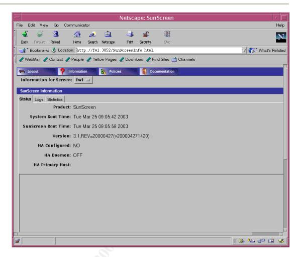
Select the "Policies" tab in the top blue strip. This will present the main Policy Window that is where most configuration steps are initiated. The "Information" tab provides GUI access to the firewall's log files. The log files may be accessed and used with other scripts for analysis from the command line interface.
