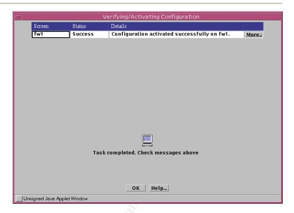
The above screen shows the successful compilation and activation of the policy. In a multi-firewall design with Central Management, there will be a line for each screen or firewall.
