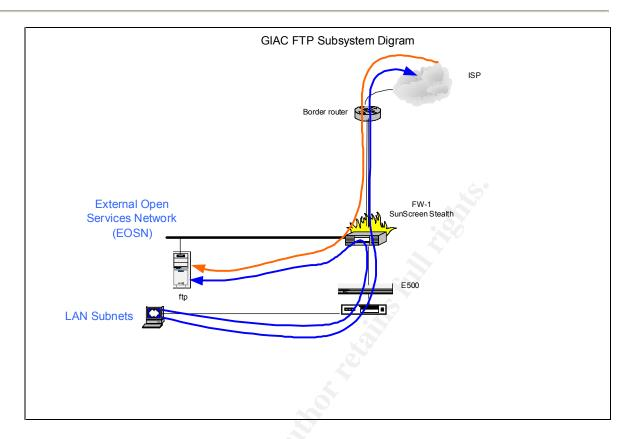
At GIAC Enterprises ftp is used primarily as a means to transfer mail attachments that exceed the size limits imposed by the internal mail system. Consequently, both external and local users must access to the ftp server. Only IT employees are authorized to access external ftp sites.
