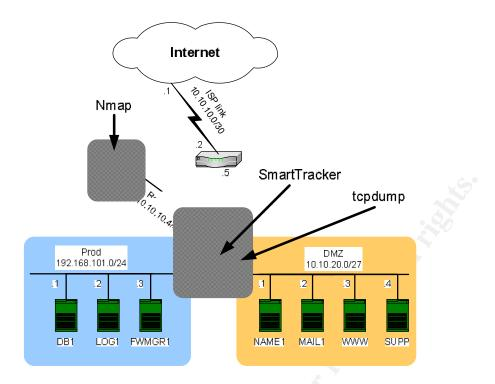
1. The audit laptop assumes the ISP router's internal IP address again for this test. Nmap is running on the audit laptop, SmartTracker on the firewall and tcpdump on the www host. Each readied for the next scan.
