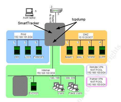
For this test, the audit laptop is disconnected and the router's internal connection is restored. tcpdump sessions are started on the internal and external firewall interfaces. SmartTracker is also readied to monitor Windows traffic.
