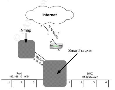
1. As mentioned above, the audit laptop assumes the internal IP address of the ISP router for this test. Nmap and SmartTracker are readied for the scan.
