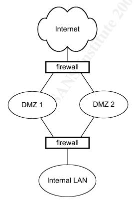
Alternate 2. Also uses a single firewall but separates the DMZ. Each DMZ will be on a separate subnet and off a separate NIC on the inside of the firewall. One DMZ will satisfy the public services and the other DMZ will handle VPN / private services.
