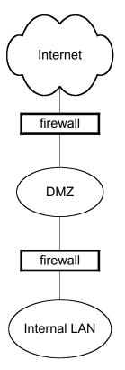
Alternate 1. A single firewall allowing all approved services into a single DMZ. This DMZ will offer services to the general public as well as VPN connections to partners. This is then separated from the Internal LAN by a second firewall. The firewalls will be different products on different Operating Systems.
