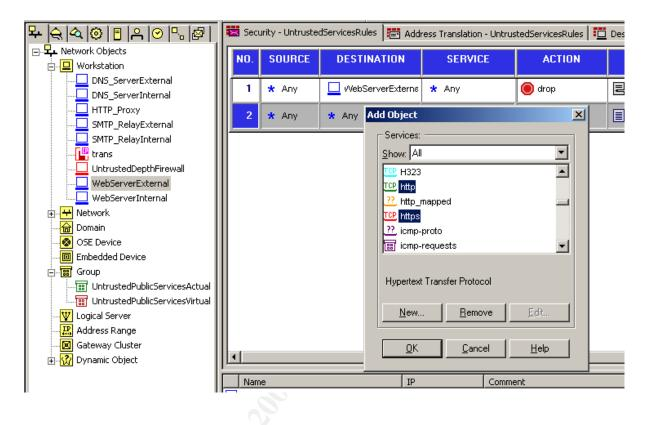
Now we define an action that the firewall is to carry out in terms of the source, destination and service. We want everyone to be able to connect, so we accept these connections. The tracking is used to create a log entry relating to the transaction. This should be used intelligently, as logs can fill quickly. The other boxes are somewhat self-explanatory. Use the comments box to keep track of the purpose of the rule. Our final rule appears as:
