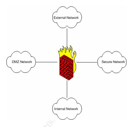
Any system on any given network segment must pass through the firewall to communicate with a system in a different network segment. This means that the a set of firewall rules must allow network traffic into the respective network segment, as well as allow the communication out of the network segment in cases of the DMZ and Secure networks.
