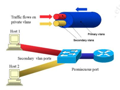
In a PVLAN, promiscuous ports are called the primary VLAN, while community and isolated ports are called secondary VLANs. A PVLAN will only have one primary VLAN, but may have several secondary VLANS.
