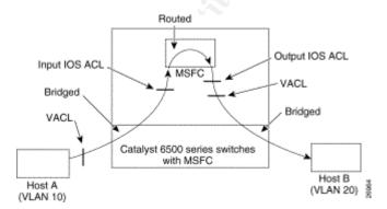
For routed/Layer 3-switched packets, the ACLs are applied in the following order:
