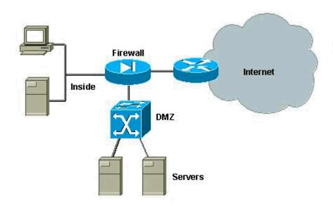
While no two DMZs are alike, for this example we will assume that the DMZ servers do not need to communicate with one another. Using the defense in depth principles, we can harden the border router ACLs, tighten firewall rules, and place NIDS in the infrastructure. However, in a typical environment, without PVLANs and VACLs, if one of these servers is compromised, an intruder would now be free to start launching attacks against other hosts on the same network space.
