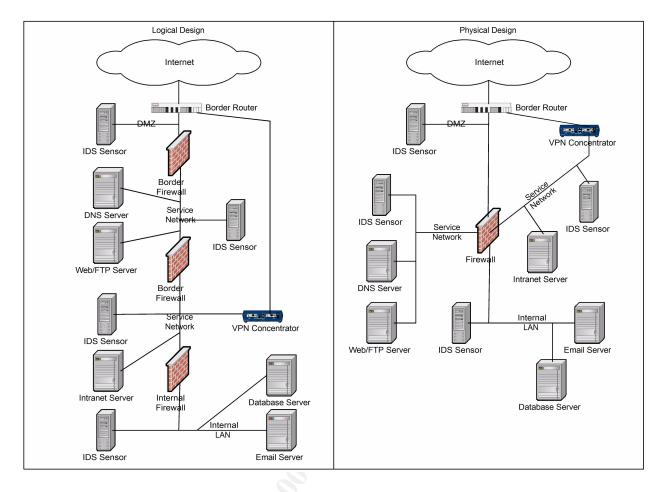
As in the first two designs, the border router is the first line of defense and filters known bad traffic. The border router does not need special configurations simply because it is at the corporate office.
