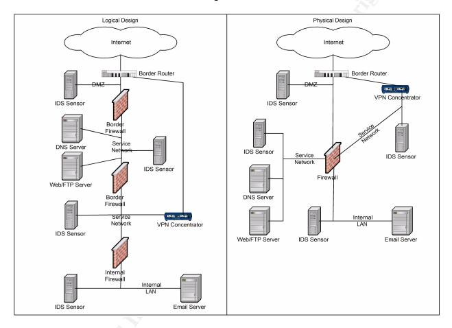
Similar to the first design, the border router is the first line of defense and will filter known bad traffic. In this design, more traffic will be allowed past the border router to support sales operations, but the traffic will still have to pass the border firewall.
