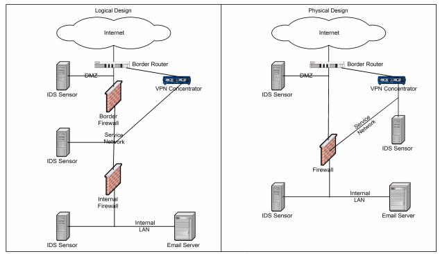
Through this design, known bad traffic can be filtered at the border router, providing the first line of defense. Traffic that passes the border router will then have to pass the border firewall. The reasoning behind having a border firewall and a service network is that many firewalls do not adequately check encrypted VPN traffic. By terminating VPN connections within the service network and not the internal LAN, all VPN traffic can then be decrypted and scanned by the internal firewall.
