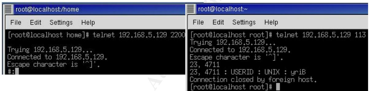
**Figure 11: telnet on tcp ports 2200 and 113**
