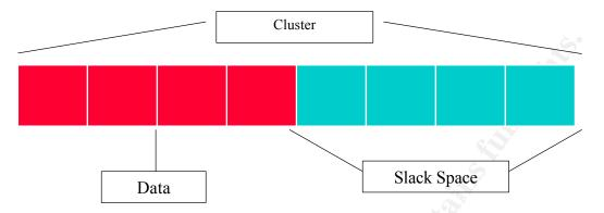
Using this concept, if a cluster is filled with data, and then the cluster is only partly overwritten, the data in slack space is recoverable. It can be viewed and recovered using a tool such as Norton Utilities DiskEdit, but is more efficiently recovered using forensics' tools such as NTI's GetSlack and Guidance Software's EnCase.
