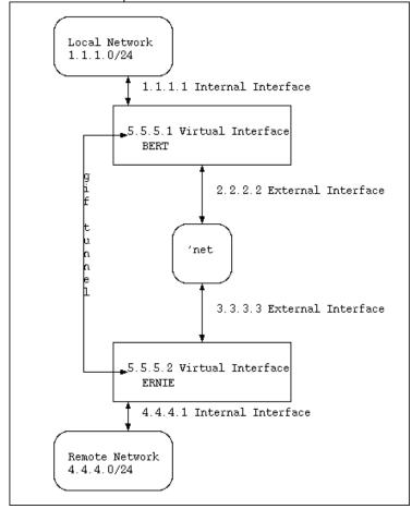
The gif tunnels external end-points are 2.2.2.2 and 3.3.3.3 and the internal end-points are 5.5.5.1 and 5.5.5.2.
