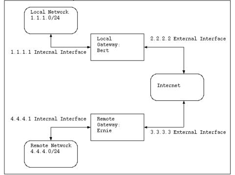
The initial goal is to have the two gateways automatically route and encrypt traffic between the two networks. I'll demostrate the NAT'ing after completing the initial goal.
