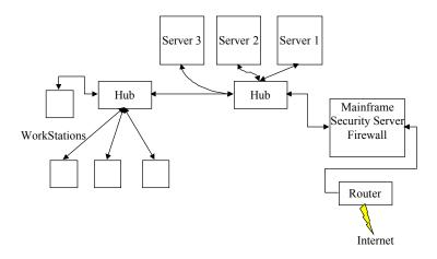
Diagram B shows how the mainframe can become the security gateway for the network infrastructure for any corporation that has a mainframe computer. The best way to look at this is by analyzing the six questions from the previous section.
