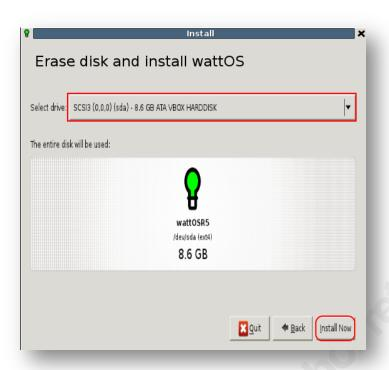
Install – Erase disk and Install wattOS5. Select 'SCSI3 (0,0,0) (sda) – 8.6 ATA VBOX HARDDRIVE'. Click 'Install Now'.
