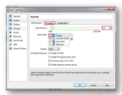
Under 'System – Motherboard' tab, uncheck 'Floppy' from Boot Order. Set Base Memory to '512 MB' as a minimum. Note: If your system has at least 4 GB of memory, change this to 1024 MB. Click 'System - Processor' tab.
