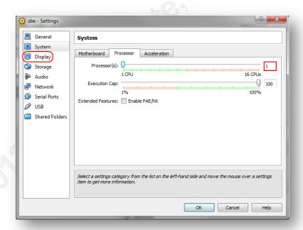
Under 'System – Processor' tab, select number of processor(s). Again, if your system supports it, select an appropriate number of processors. Click 'Display' tab on left.
