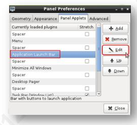
Right-click on LXpanel bar, select 'Add/Remove Panel Items'. Highlight 'Application Launch Bar' just below Menu/Spacer entries. Click on 'Edit' tab.
