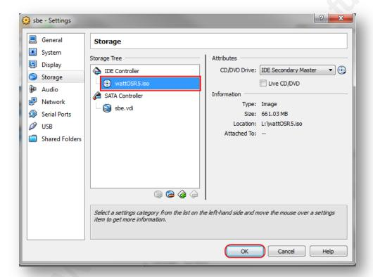
Under 'Storage', click drop-down CD icon next to CD/DVD Drive, and choose 'Choose a Virtual CD/DVD Disk file' and select 'wattOSR5.iso' that has been downloaded and saved (http://www.planetwatt.com/wattiso/wattOSR5.iso). This will complete the configuration of the VM at this stage. Click 'OK'.
