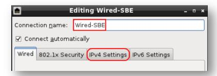
Under 'Wired' Network Connections, Click 'Add', Enter Connection Name: 'Wired-SBE'.
