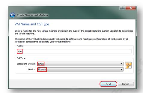
Create New Virtual Machine - VM Name and OS Type. Enter 'sbe' for Name, select 'Linux'/Ubuntu' for Operating System/Version. Click 'Next'.
