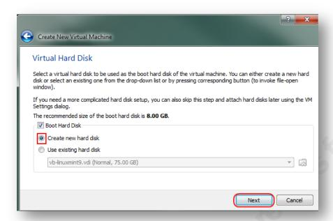
Create New Virtual Machine – Virtual Hard Disk. Select 'Boot Hard Disk – Create new hard disk'. Click 'Next'.
