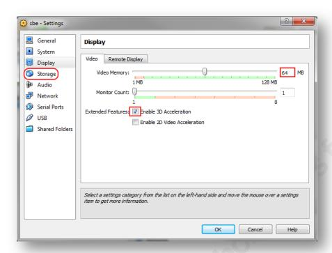
Under 'Display - Video' tab, select '64 MB' for Video Memory. Check 'Enable 3D Acceleration' under Extended Features. Click 'Storage' tab on left.
