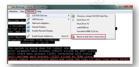
Release 'wattOSR5.iso' from CD/DVD Devices by selecting 'Remove disk from virtual drive'. Hit 'Enter' to continue reboot.
