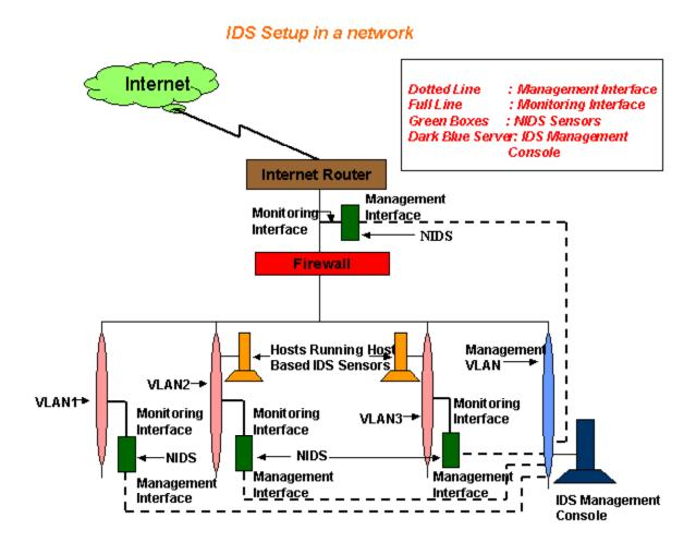
Picture1: Deployment of IDS Sensors and Management Console in a network
