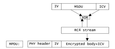
The 802.11 standard specifies that the ICV is to be calculated by a standard CRC, just like the frame check sequence (FCS) which is used in frames that are not encrypted. If the receiver gets a packet that has an invalid ICV or FCS, the packet is silently dropped (except for the encrypted 3rd packet of a Shared Key authorization request.)
