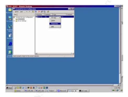
After selecting properties and under the general tab, there is an option that allows the administrator to change the encryption level that is being used.
