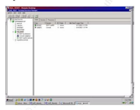
This utility will show the administrator the current users who are connected to the Terminal Service and their status. As shown in the above screenshot, user jshively is logged into Terminal Service via RDP-Tcp#26 and has been connected since 3:13 p.m. Notice the column labeled "state" displays active. This indicates that this is an active session that is currently being used. If the session was disconnected the column labeled "state" would display disconnected.
