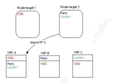
This topology is known as a hub and spoke, with the OSS VRF as a hub. The spokes can speak with the hub, but not between each other.
