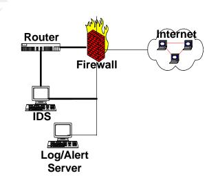
In this example the router and firewall work together to monitor and control inbound and particularly, outbound traffic. Note how the IDS is connected to the router and firewall to cover off all of the monitoring requirements.
