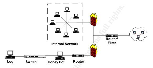
A DMZ is created for the honey pot to reside in. The router and firewall are still combined to control all traffic in and out of the network.
