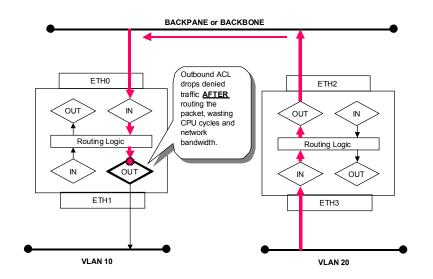
To provide the control desired, ACLs would need to be applied to ALL inbound interfaces on ALL routers connected to the company network. Although this is a desirable goal, there just was no practical way to accomplish such a feat in the time frame allotted and with the resources available. Consequently, we had to settle for applying ACLs to both the inbound and the outbound interfaces for the 10 VLANs remaining in our scope. Twenty ACLs were needed as shown in the table below:
