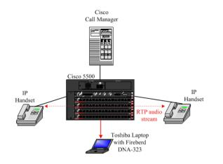
If configuration access to the switch was unavailable other techniques such as ARP spoofing could have been used to ensure that the tool captured the RTP packets. ARP spoofing is a technique used by hackers to alter the normal flow of IP packets. The technique involves generating a spoofed ARP response packet in response to a valid ARP request packet. This process enables the hacker to direct the flow of IP packets through a compromised workstation from where the packets can be captured.
