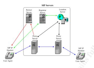
The size and scale of a SIP network will dictate the number of servers required for an implementation. However, it should be noted that for small implementations a number of services can exist on the same physical server.
