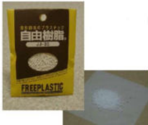
Fig. 2. Freeplastic used for fingerprint mold
