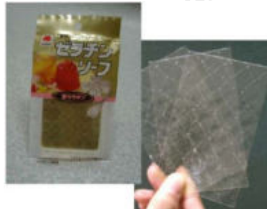
Fig. 3. Gelatin sheet used for gummy finger
