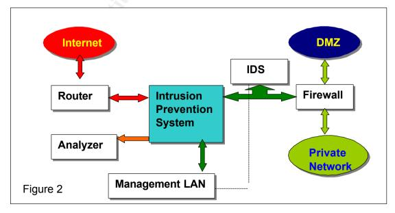
Enterprise to Internet connectivity example deploying an Intrusion Prevention device -
