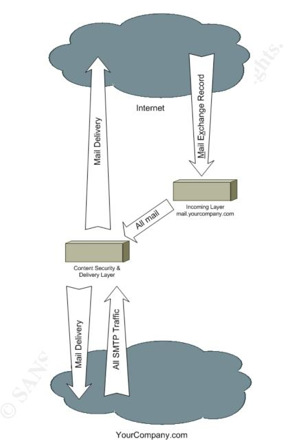
In this scenario we have one server handling the incoming layer and one server handling both content security and delivery layers. For this example, we are going to assume the content security layer is running a product that will use sendmail to deliver the filtered mail. SCENERIO TWO: Three-tiered design separating the three layers on to separate servers.
