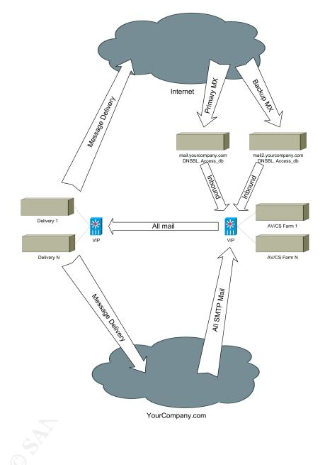
SECENERIO THREE: In this case all layers are separated and we have expanded the content security layer into two separate pieces to demonstrate how multiple content security vendors could be used together.
