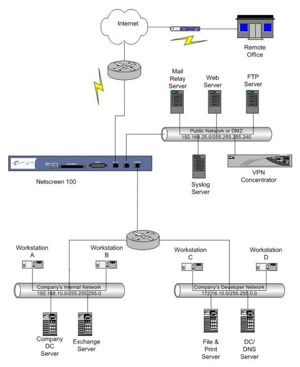
In the previous diagram, we placed the Netscreen 100 firewall behind the outermost router. This router connects our ISP and our internal network. Since we had a web server, a mail server, and a VPN device, we wanted to place those devices within the DMZ. The rest of our systems would reside on our trusted network such as Domain Controllers and File & Print servers.
