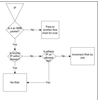
From the flow charts, they were able to identify where they would place limiter devices such as firewalls. It was also evident where they would install sniffers and IDS. In addition, Policies were easier to review and implement based on a clear understanding of how traffic moved into and out of the network.
