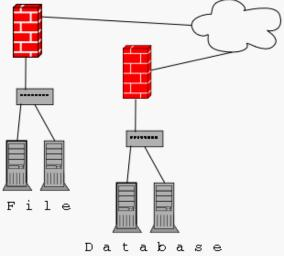
In this configuration, rules are optimized by separating them onto multiple Hogwash systems to increase performance and by grouping servers according to the services offered to match the rules.
