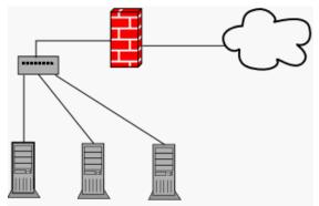
In this setup the Hogwash system is attached to the network where the servers used to be and the servers are either connected to a hub into the second Hogwash NIC or multiple NICs can be used in the Hogwash system.
