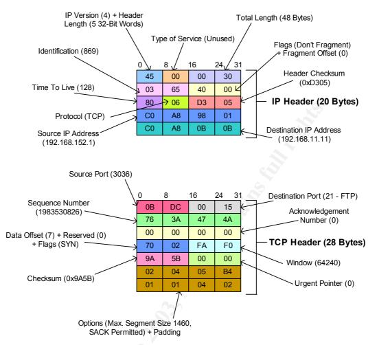
Note that there is no TCP data segment. It is simply a connection request. The first fragment involved in the attack will carry the first 16 bytes of the TCP header. The following changes will be made to the IP header:
