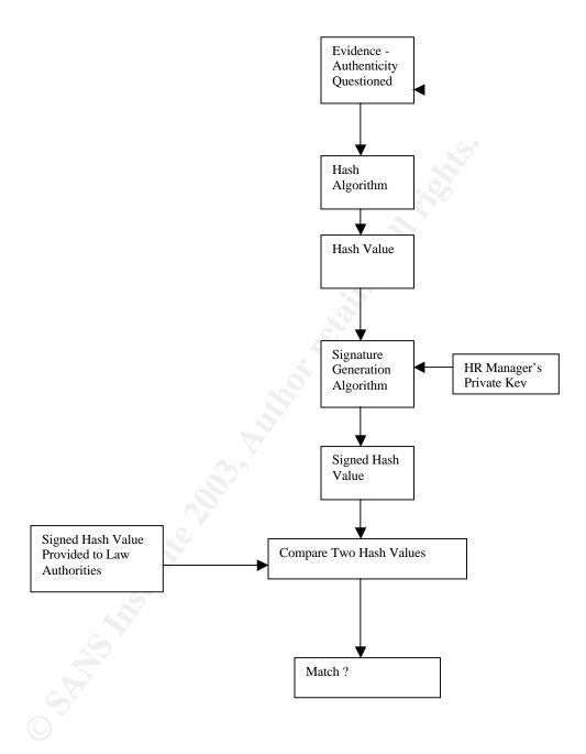
Figure 2: Validating Evidence Integrity and Authenticity
