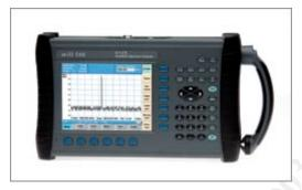
Spectrum analyzers are high-end devices that monitor the strength of various frequencies in the RF spectrum. Their use is not trivial, they are expensive and they need to be operated by qualified personnel. [willtek1]
