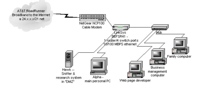
This diagram shows one possible arrangement to take advantage of the segregation available with a router. With all defaults in place (including no DMZ), the "Sniffer" box has almost nothing to watch. The combination of switching and routing, with a browser-based configuration GUI to set port options, reduces the network to external traffic specifically addressed - and by default returning from established connections only.
