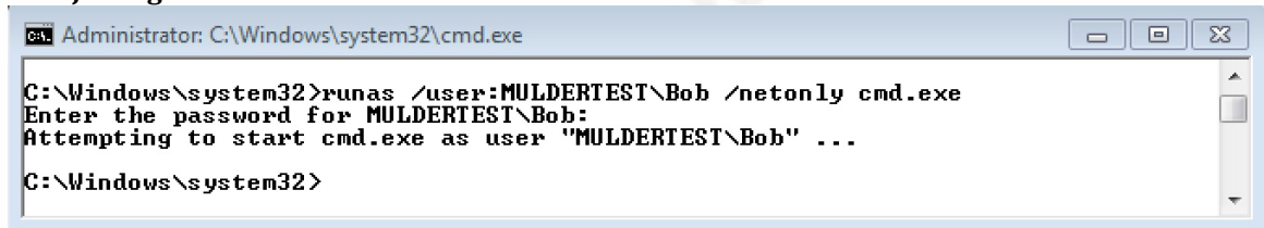
Figure 14: Injecting credentials into LSASS
