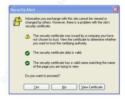
Once the two SSL tunnels have been established, the packets from *PC1* are available in cleartext to *Sniffer*, and Active Dissector can extract usernames, passwords, and data as easily as with any normal HTTP traffic before forwarding the packets to the real web server.
