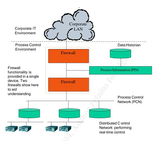
To provide a further layer of segregation , data would be pushed from the Process Control N etwork to the data historian on the PIN (DMZ). Users would then pull data from the historian to applications on the cor porate network. This data flow is illustrated below.
